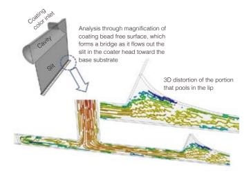
Coating bead flow analysis for slots with microfiber linkage
