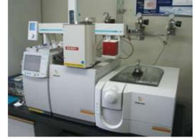
Pyrolysis gas chromatograph mass spectrometer
