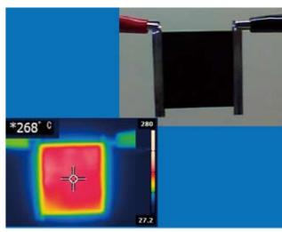
Ultrathin, high-temperature CNT membrane heaters that feature good temperature response.
