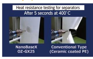
Nonwoven fabric separators with high heat resistance help ensure improved battery safety.
