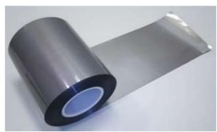
These thin nonwoven fabric sheets are used in EM shielding materials.
