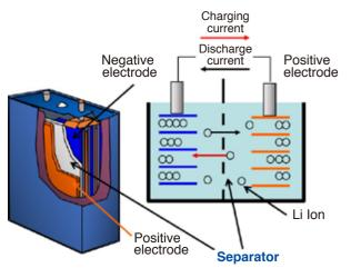
Structure of the lithium-ion battery
