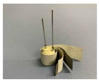
Photo of capacitor disassembly (the yellow sheet is a separator.)
