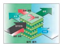
Mechanism of a total heat exchange element
